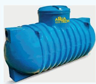
AQUA TECH Septic Tanks comes with "3 Chamber Baffle Design" system. This ensures a high degree of settlement and sedimentation, thus providing a low level of suspended solids, suitable for discharge into any underground soak-away system.
